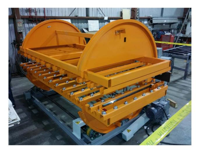
The TRM-180 Barrel Turner is a manual version of the Barrel Turner with two non-motorized roller conveyors or two transfer ball tables nested into a cylindrical enclosure that rotates on its own axis. The system features powered rotation of the assembly, but the infeed and outfeed of the panel are done manually by the users.
