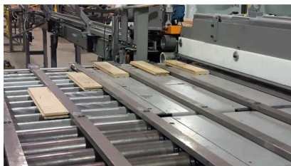
GPS - CROSS TRANSFER ROLLER CONVEYOR
