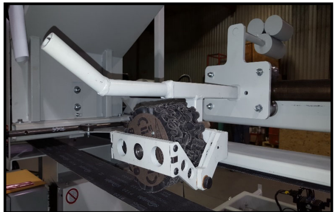
Contact Wheel Assembly with Corrugated Stacked Disks
